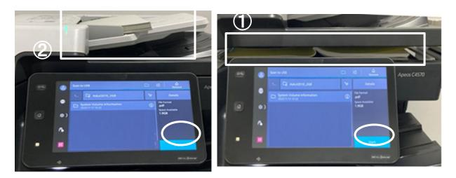
Select the folder where you wish to save the scanned document  $\rightarrow$  press [Start] When the scanning is complete, press [Remove] $\rightarrow$  remove your USB
