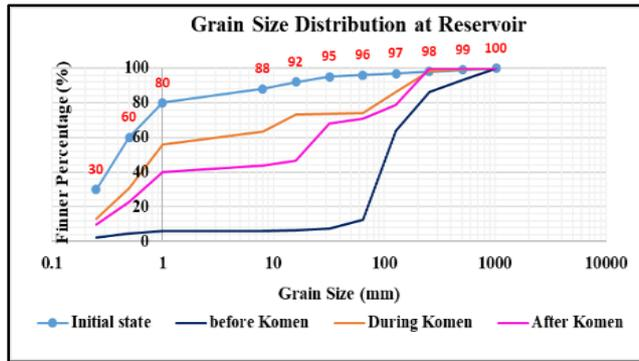
Figure 5 shows the grain size distribution results at the reservoir for Case 3. In this case, we consider the large amount of fine-grain 80% and coarse grain 20% as input data, and the blue line is the initial state of sediment grain size distribution. We can see all of the fine-grain sediment results are smaller than the initial state. On the other hand, coarse sediment % is greater than the initial state into the reservoir location depending on sediment supply rate and high flood level.
