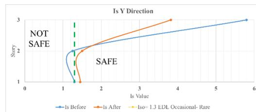
Figure 10. Retrofit with infill wall in Building 2.
