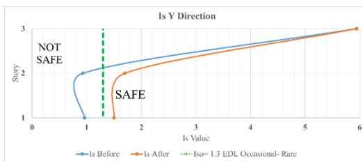
Figure 9. Retrofit with infill wall in Building 1.
