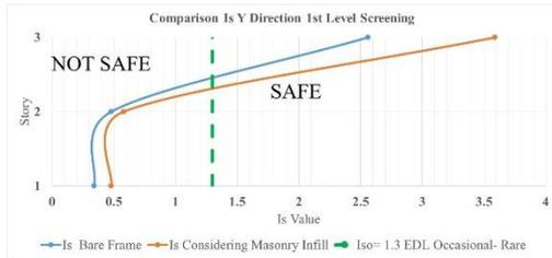
Figure 5. Comparison of bare frame and frame with Reinforced masonry wall in the First Level Screening, building 1.
