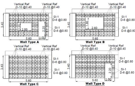
Figure 3. Details of Infill Masonry Walls for Building 1 and 2.
