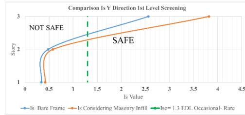
Figure 6. Comparison of bare frame and frame with Reinforced masonry wall in the First Level Screening, building 2.
