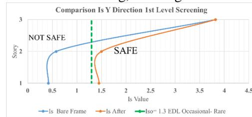
Figure 8. Retrofit with infill wall in Building 2.
