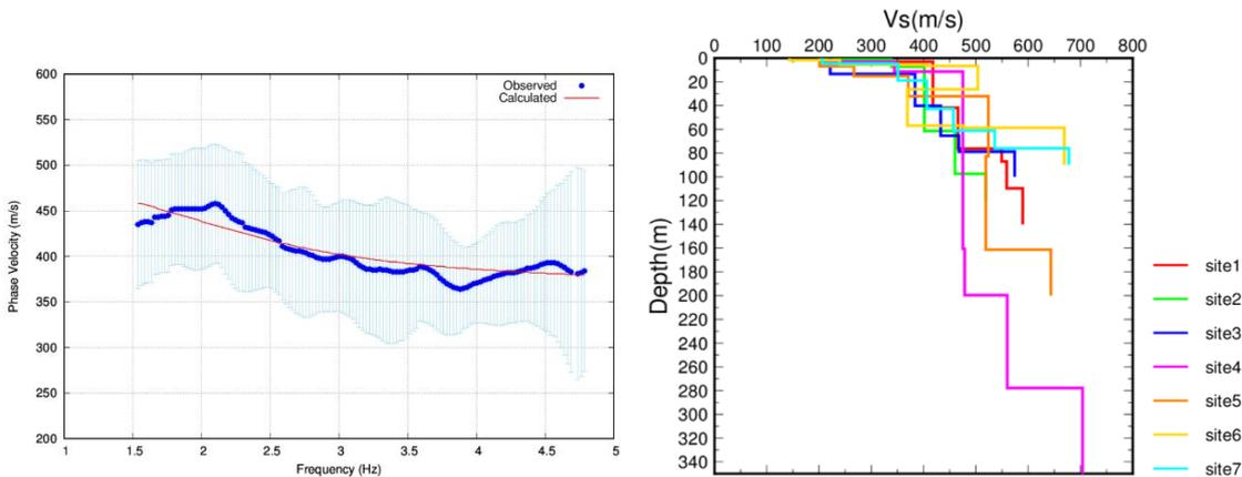
Figure 3. Left) Comparison between observed and calculated dispersion curve at site 2. Right) The resulted  $V_s$  structure models for the 7-sites in Ismailia city.
