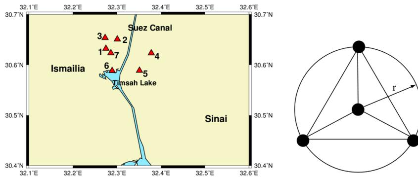
Figure 1. The location of microtremor array observation sites in Ismailia city (left). Circular array configuration with four sensors (right) (after Okada, 2003).
