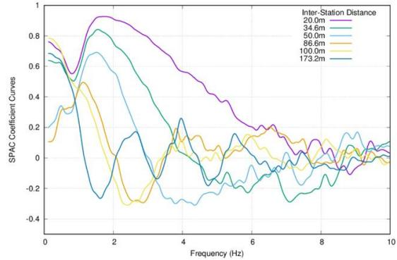
Figure 2. The obtained 6-SPAC coefficients of large, medium, and small arrays at site 2.
