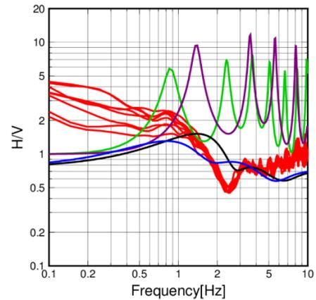
Figure 5. HVSr for the eight-sensors records (red curves) with the site amplification factor of inverted Vs-structure (purple curve) and that of the modified Vs-structure (green curve), and theoretical HVSr of inverted Vs-structure (black one) and that of modified Vs-structure (blue one) at site3.
