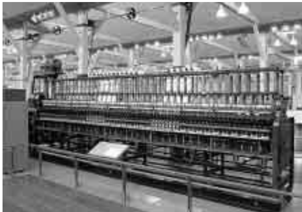
Modern Ring spinning frame made by Platt, U.K., 1896.
